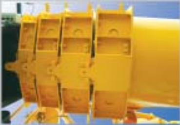
独特的吊臂对中装置 Specific boom aligned devices
