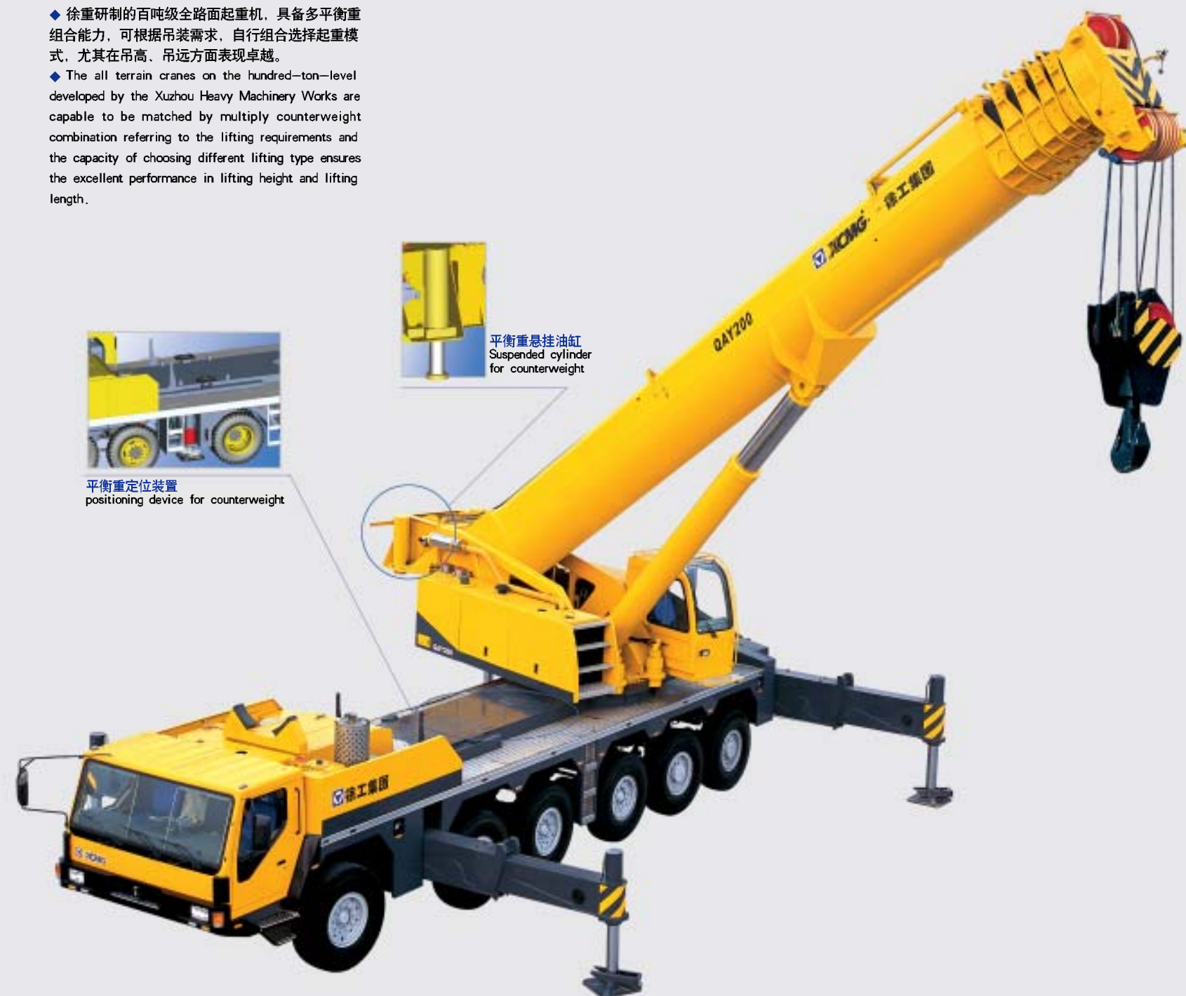
平衡重自装卸 Self-assembly of counterweight
