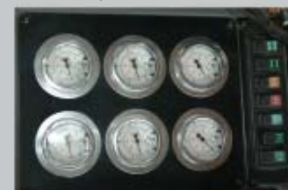
油气悬挂压力表 Pressure gauge of hydro-pneumatic cylinder
