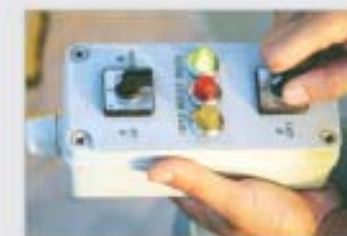
平衡重遥控器 Counterweight remote controller
