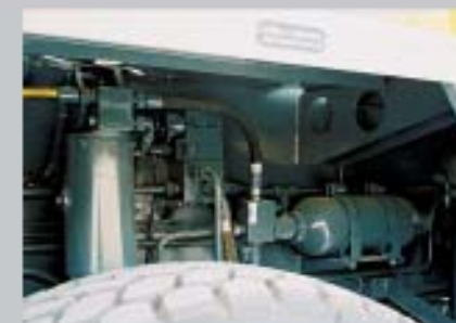
悬挂油缸 Suspended cylinder
